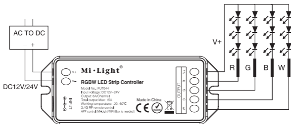
Controller connect to RGBW LED strip diagram
